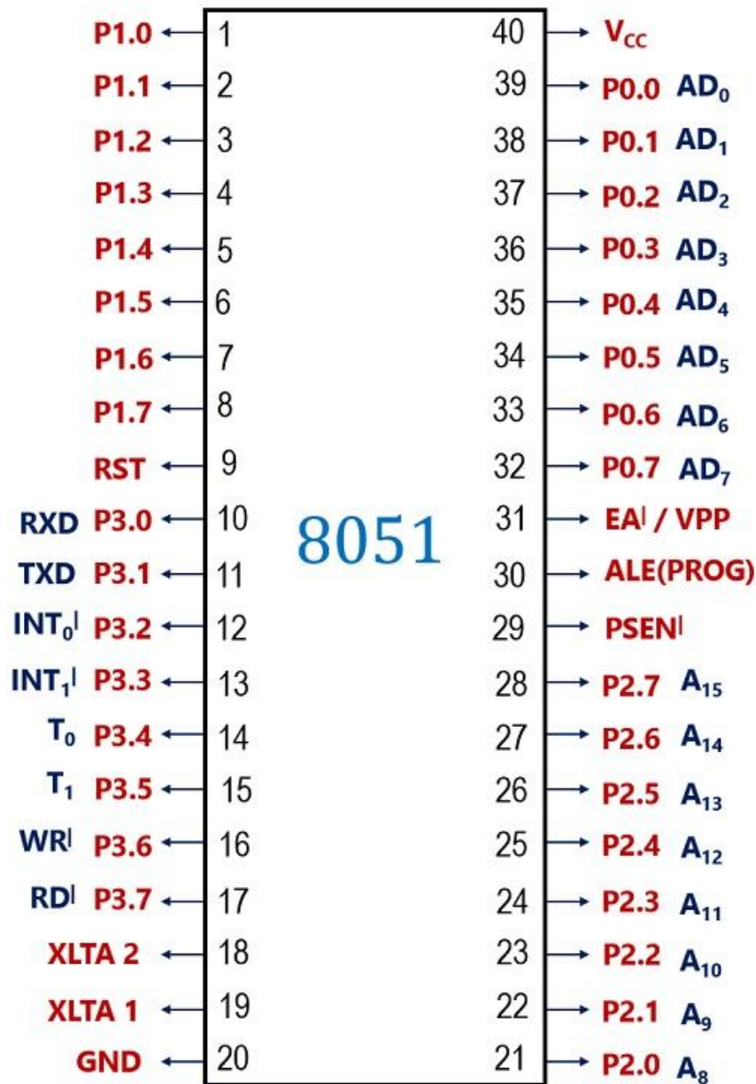
Pin diagram of 8051 Microcontroller
