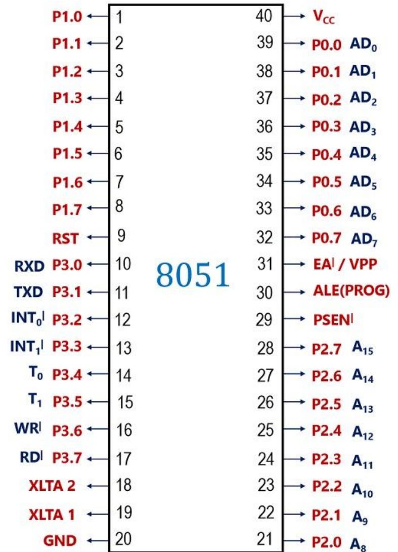
Pin diagram of 8051 Microcontroller
