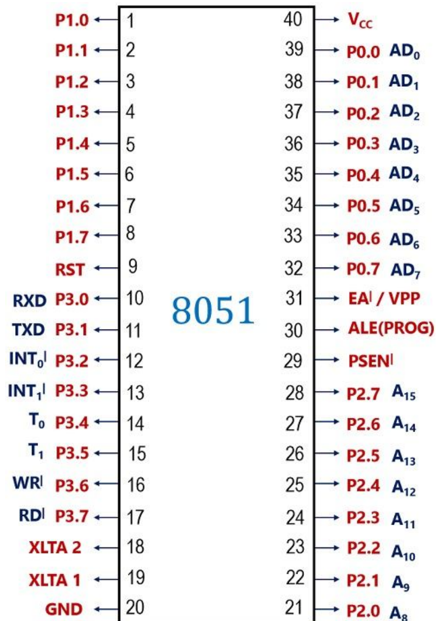
Pin diagram of 8051 Microcontroller
